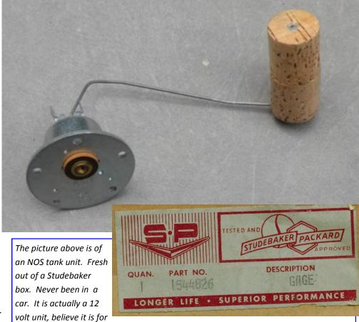
a '58. Not sure how long that pristine cork would survive with today's fuel. But even being unused, it appeared to have contact problems and might have to be cleaned before it can be used. It is for sale as I have no plans on acquiring any 12 volt Studebakers.
