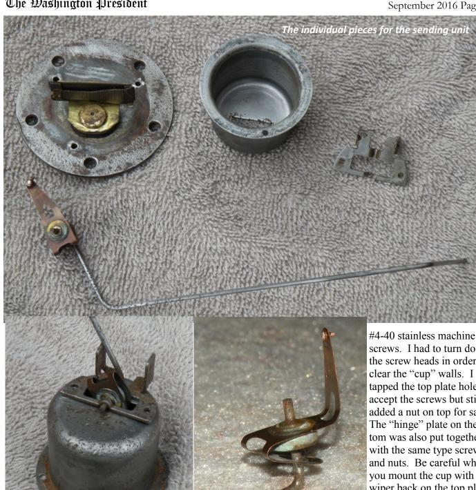
The cup with the arm and hinge plate (Rivets already removed)
